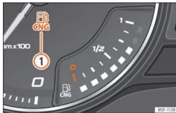
Fig. 133 Analogue instrument panel: natural gas gauge
