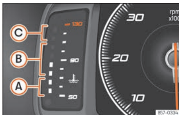
Fig. 135 Digital instrument panel: engine coolant temperature display.
