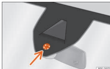
Fig. 157 Rain sensor sensitive surface
