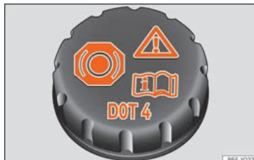
Fig. 65 Engine compartment: brake fluid reservoir cap.
