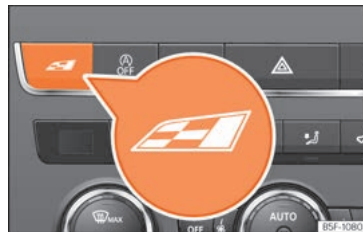
Fig. 282 Centre console: Cupra Drive Profile button.
