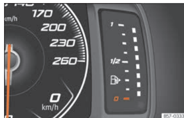
Fig. 132 Digital instrument panel: fuel gauge.
