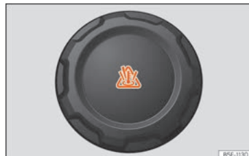
Fig. 64 Engine compartment: coolant expansion tank cap.
