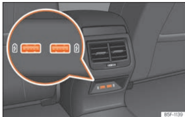
Fig. 248 Centre console, rear section: USB connectors.
