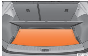
Fig. 176 In the boot: fitting the rear shelf.
