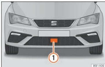
Fig. 266 On the front bumper: radar sensor.
