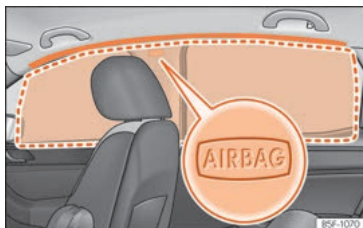
Fig. 34 Location of head-protection airbags.
