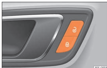
Fig. 5 Driver door: central locking switch.
