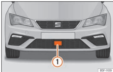
Fig. 271 On the front bumper: radar sensor.
