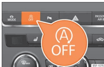
Fig. 262 Centre console: Start-Stop system button.
