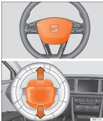
Fig. 26 Driver airbag located in steering wheel.
