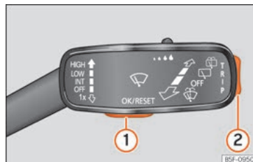
Fig. 136 Windscreen wipers lever: control buttons.
