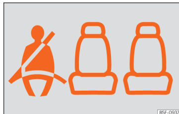
Fig. 92 Dashboard: right rear seat occupied and corresponding seat belt fastened display.
