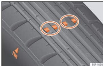
Fig. 313 Tyre profile: tread wear indicators.
