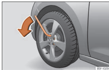
Fig. 77 Wheel: loosen the wheel bolts.
