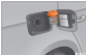
Fig. 61 Fuel tank flap with tank cap attached.
