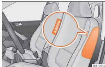
Fig. 32 Side airbag in driver's seat.
