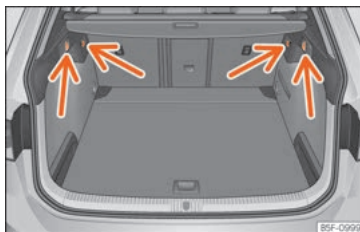
Fig. 188 In the boot: retaining hooks (LEON ST).
