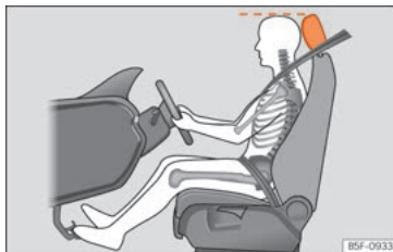
Fig. 88 Correct head restraint position for the driver.
