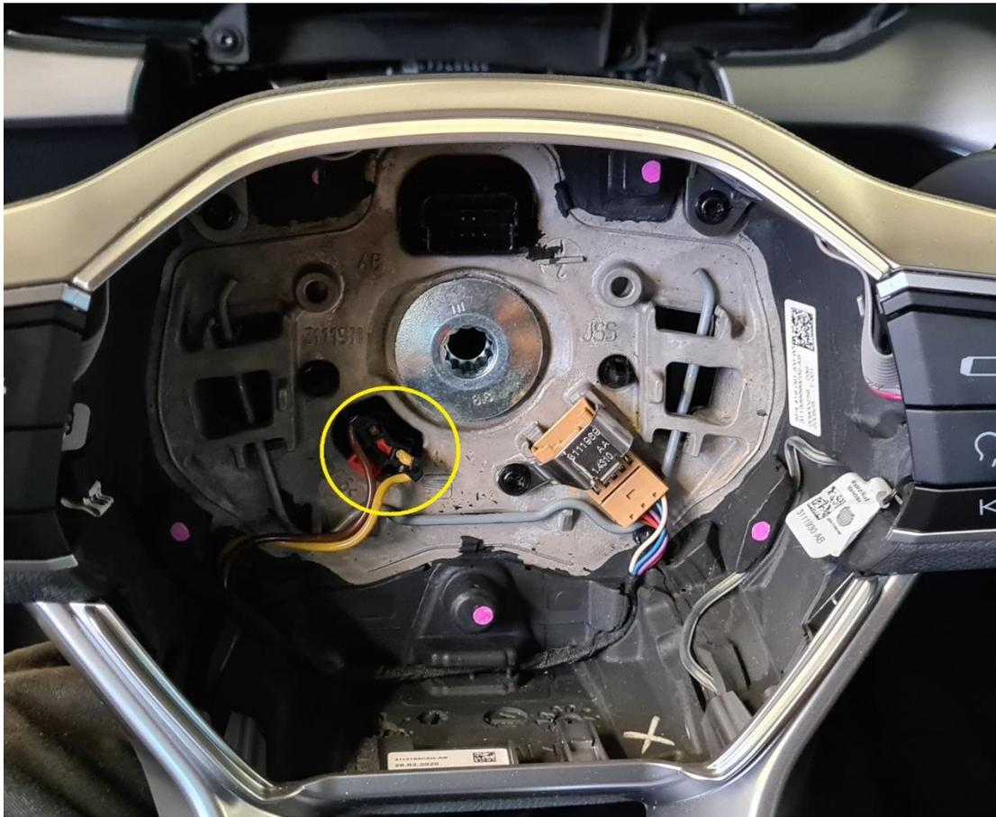
**Step 9:** Get a M12 Multitorx and loosen the center bolt off the steering wheel. ( don't remove it complete because you have to need some power on the steering wheel te release it from the steering colom ) Wiggle the steering wheel when it pops a little bit loose from the steering colom and then you can remove the bolt.
