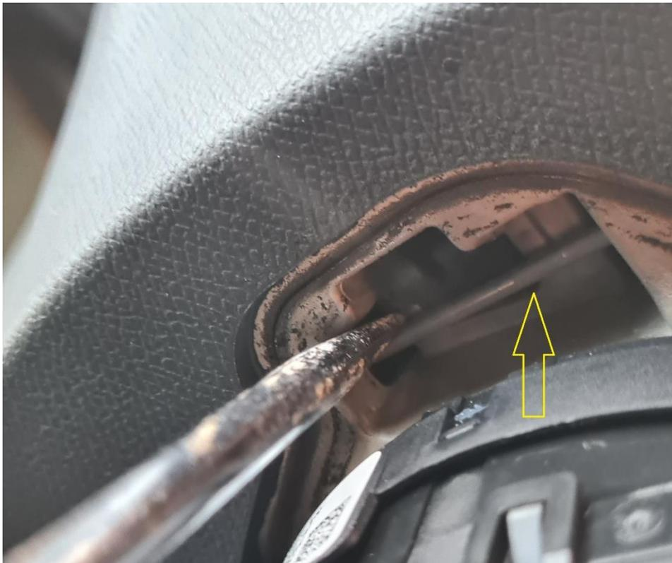
**Step 8:** Remove connector from steering wheel heating iff you have this steering wheel.
