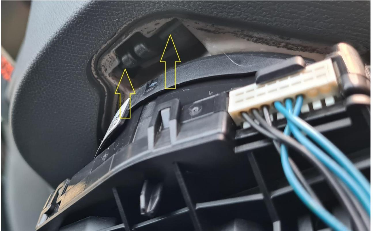
**Step 7:** Put a small screwdriver like the and unhook on side off the airbag by pulling the bar ( yellow arrow) behind the hook towards the middle off the steering wheel like this.
