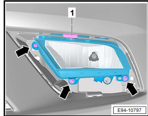
**2.1.2 Fog lights, removing and installing, FR, left side, until week 45/16**
