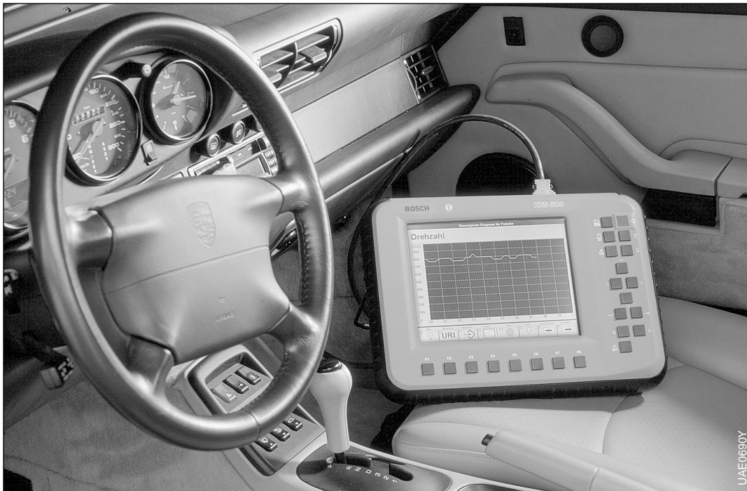
Bosch KTS 500 Motortester in use
